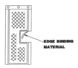
3) FOLD EDGE BINDING MATERIAL OVER CUT EDGE OF QUILTED FIBERGLASS, EQUAL AMOUNTS ON FRONT AND BACK
